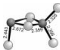
Figure 4. [\text{Ge}_2\text{Se}_5]^{4-} anion of \text{Ba}_2\text{Ge}_2\text{Se}_5 .
